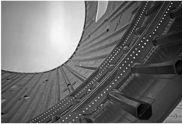
Fig. 1 Partially assembled composite fuselage section.
